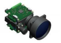
JIO-H1218X adopts the 1535nm eye-safe erbium glass laser module independently developed by Jioptik, which has the characteristics of low power consumption, small size, high precision.
